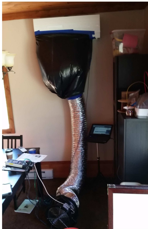
Figure 26. Ductless airflow measurement
