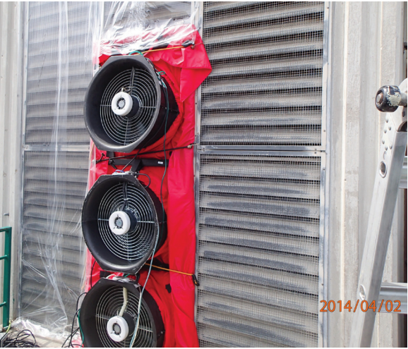
Figure 5: Airflow measurement. Crew used a calibrated fan to measure outdoor air intake airflow.
