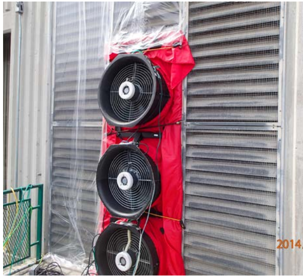
Figure 26. Blower door fans adapted to measure air intake flow using the “pressure matching” method.
