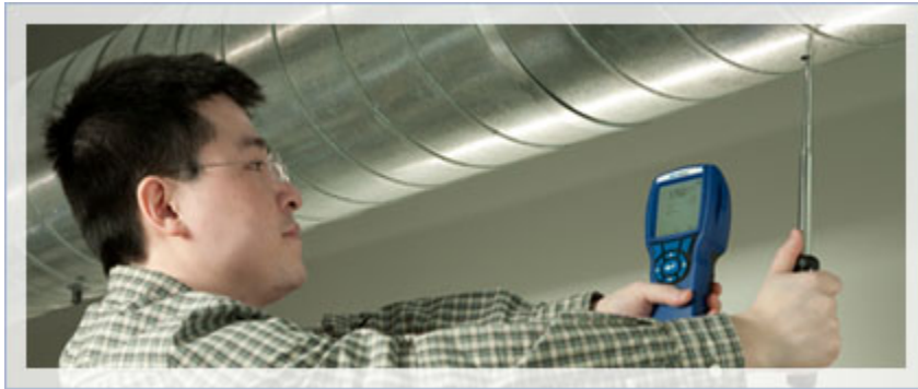
Figure 24. Measuring flow with hot wire anemometer
