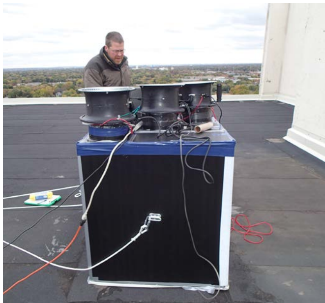
Figure 21. Customized capture box with 3 Duct Blaster fans: PRV flow is measured by matching normal operating duct pressure
