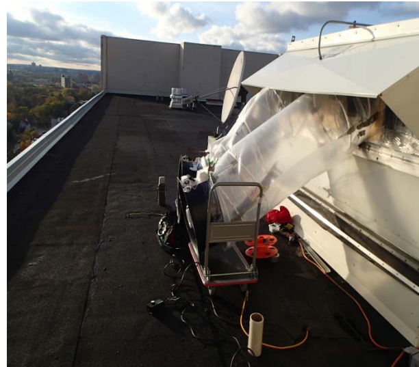
Figure 26. Blower door fans adapted to measure air intake flow using the “pressure matching” method.
