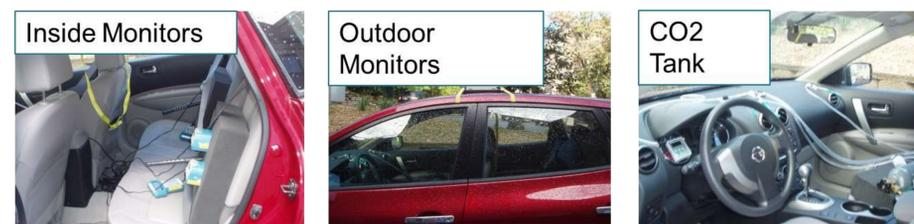
Fig. 1: PM<sub>2.5</sub> measurements were taken in the front passenger seat and two back seat locations using TSI Sidepak photometers. Injection of CO<sub>2</sub> and CO<sub>2</sub> concentration measurements were used to estimate ventilation rates.
