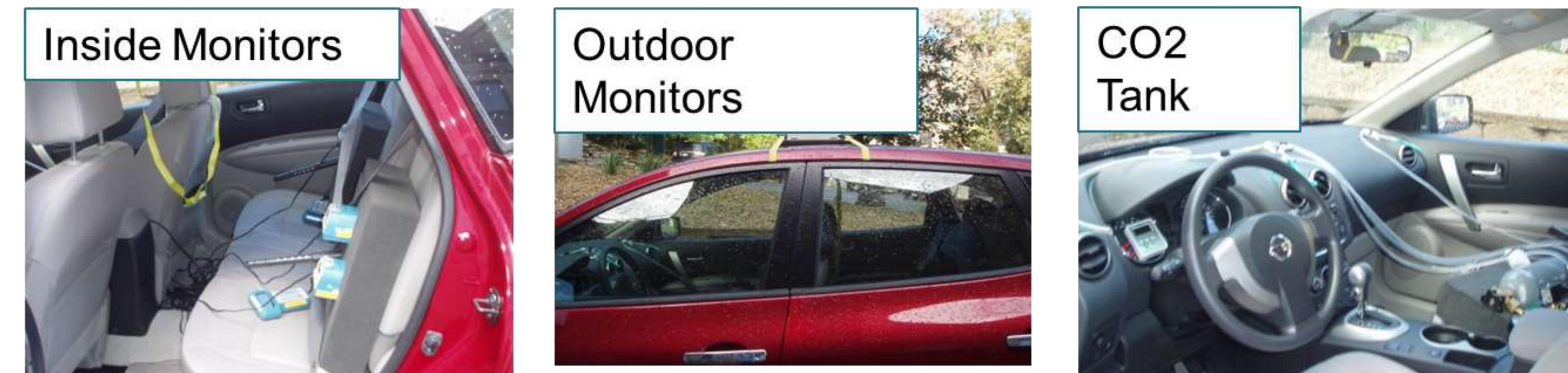
Fig. 1:  $PM_{2.5}$  measurements were taken in the front passenger seat and two back seat locations using TSI Sidepak photometers. Injection of  $CO_2$  and  $CO_2$  concentration measurements were used to estimate ventilation rates.
