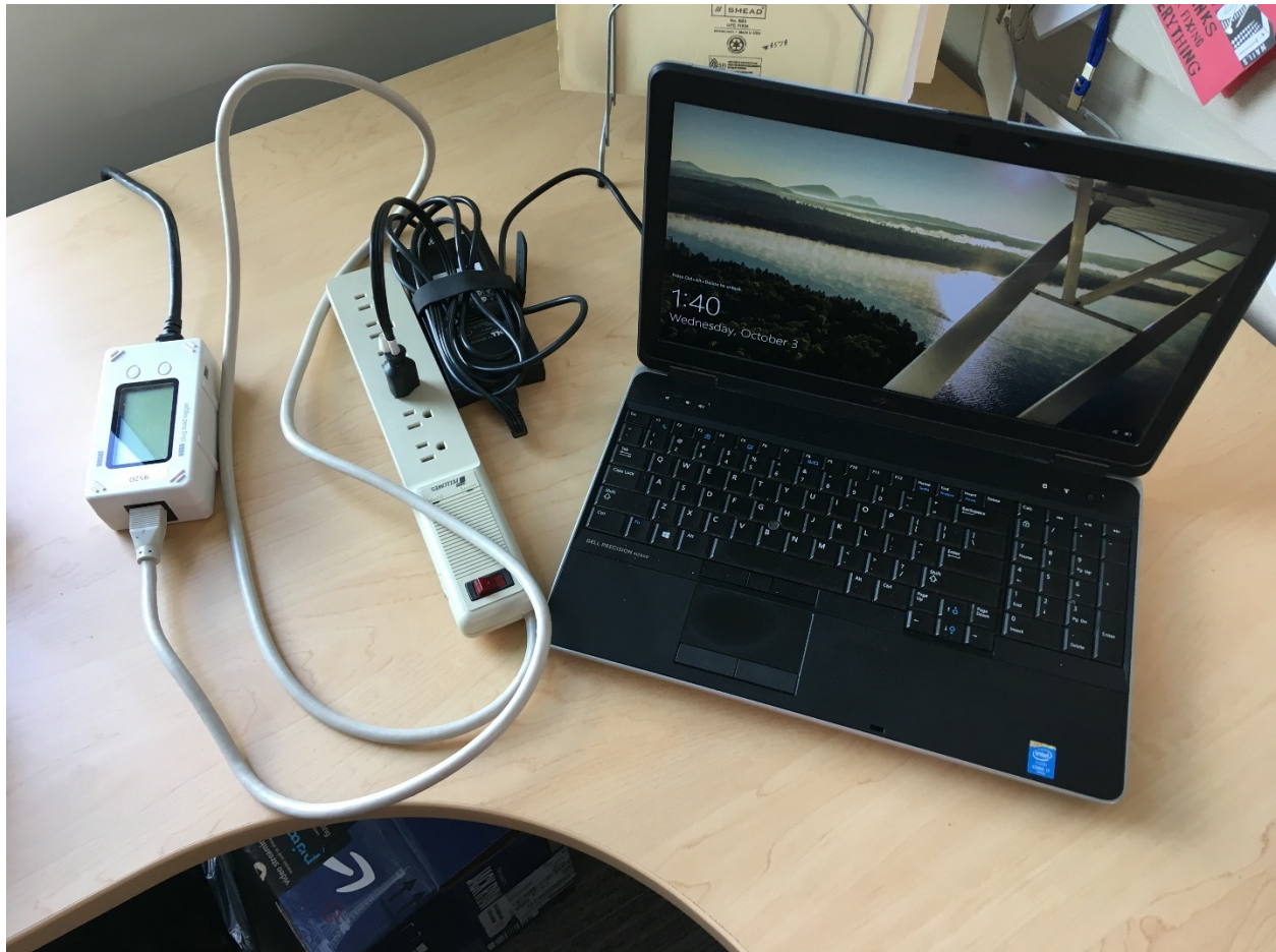
Figure 4. Metering configuration at a typical workstation.
