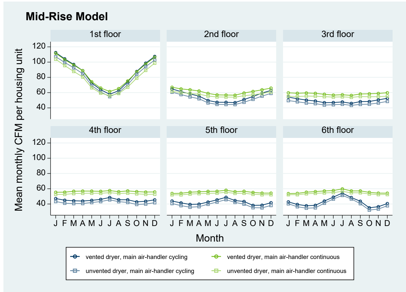
Figure 30. Monthly average CONTAM-modeled air exchange for the mid-rise model, by modeled condition and level.
