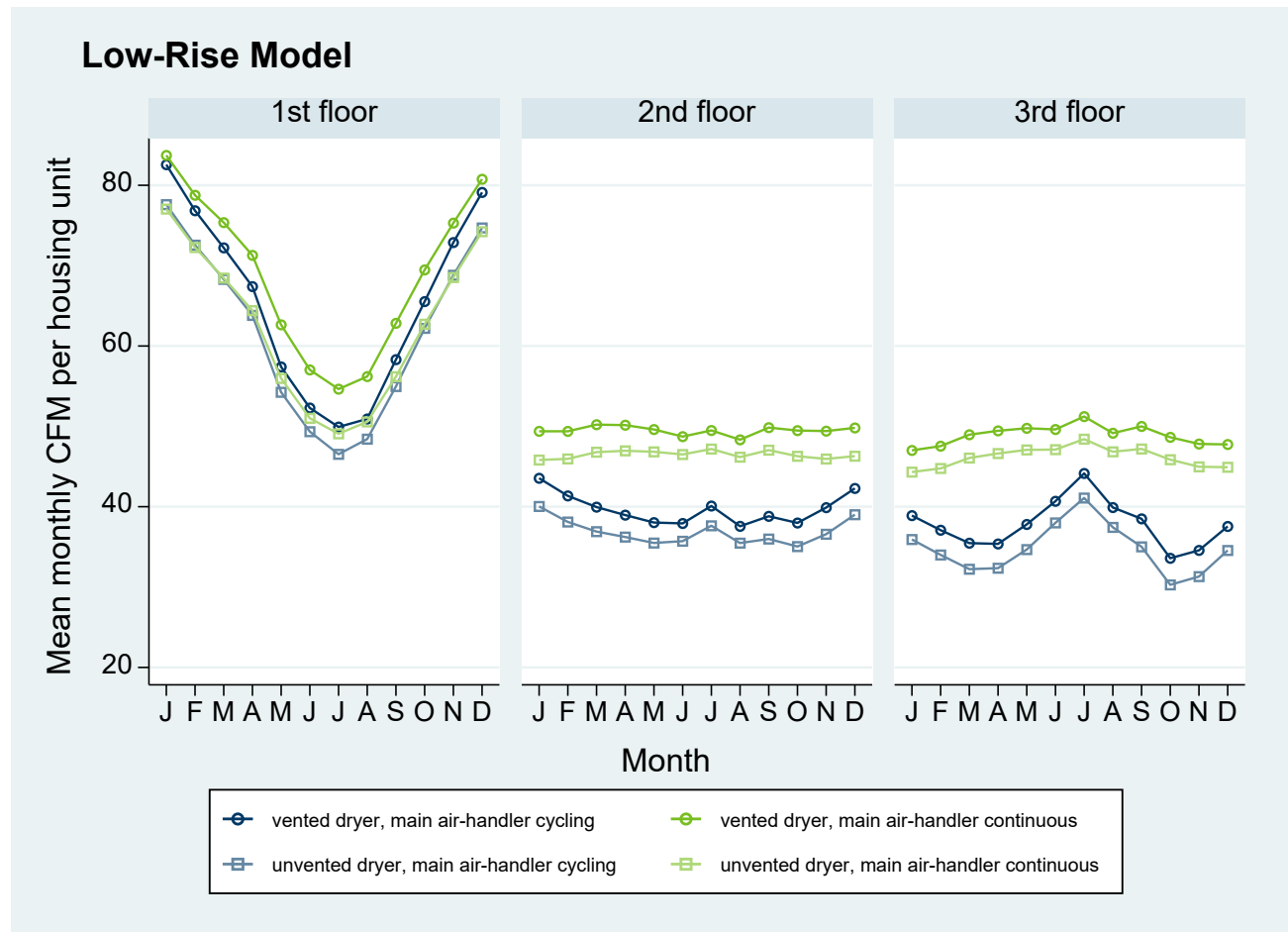
Figure 29. Monthly average CONTAM-modeled air exchange for the low-rise model, by modeled condition and level.
