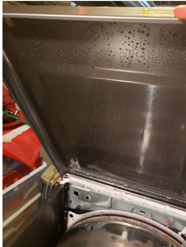
Figure 16. Moisture covering the interior of the malfunctioning heat pump dryer for Site 1.
