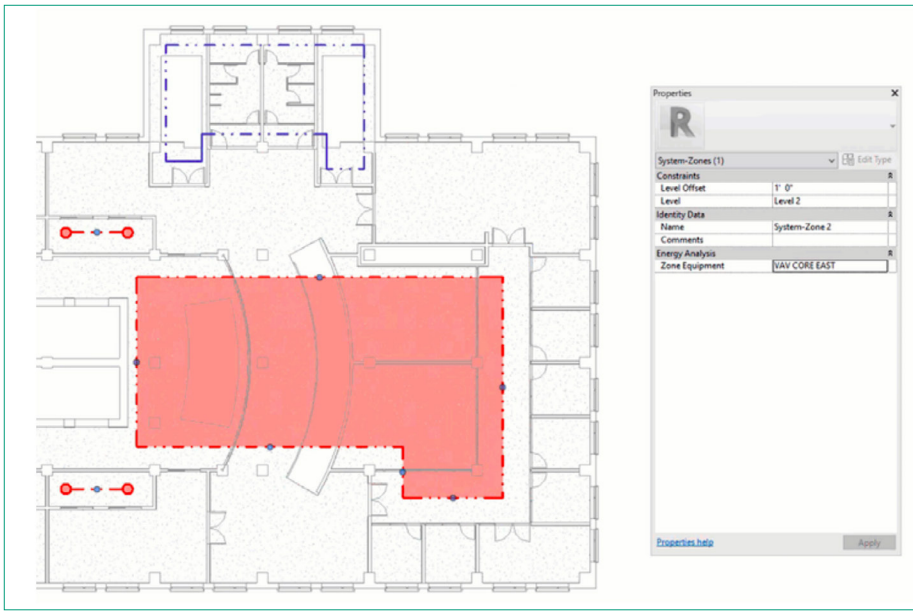
Figure 9. Systems Analysis allows Revit users to quickly group building regions into thermal zones and connect those to different types of HVAC systems. In this image, the “Core East” zone is connected to a VAV air handler. Figure courtesy US Department of Energy, Building Technologies Office.
