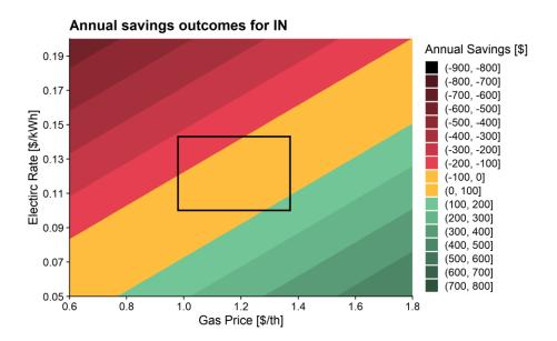
Figure 18: Contour plot of potential savings outcomes for a range of electric and gas rate combinations in Indiana
