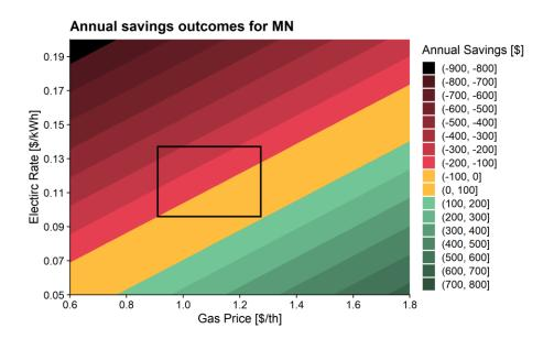
Figure 22: Contour plot of potential savings outcomes for a range of electric and gas rate combinations in Minnesota
