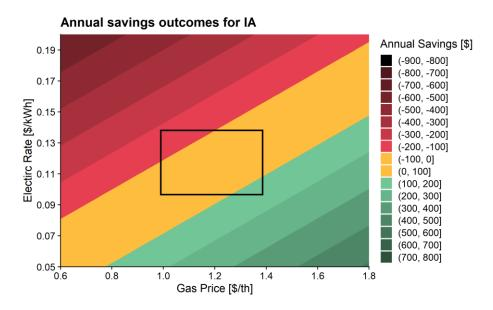
Figure 11: Contour plot of potential savings outcomes for a range of electric and gas rate combinations in Iowa.
