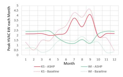
Figure 15: Peak HVAC electricity consumption for ASHPs in KS and WI vs. their baselines
