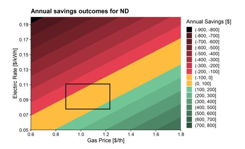
Figure 24: Contour plot of potential savings outcomes for a range of electric and gas rate combinations in North Dakota
