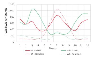
Figure 14: Monthly HVAC electricity consumption for ASHPs in KS and WI vs. their baselines
