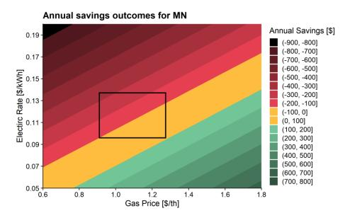
Figure 10: Contour plot of potential savings outcomes for a range of electric and gas rate combinations in Minnesota.
