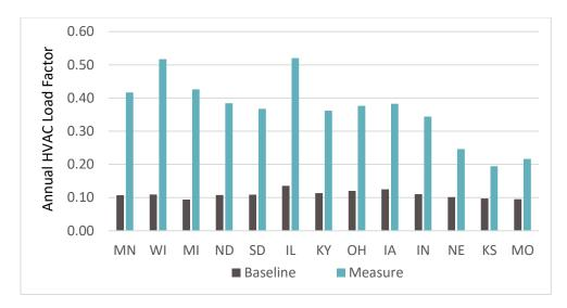
Figure 13: Annual HVAC load factor for the dual fuel ASHP measure compared to the baseline in each location
