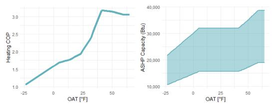
Figure 7: Cold-climate variable speed ASHP performance across heating OATs
