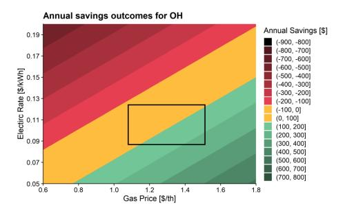
Figure 26: Contour plot of potential savings outcomes for a range of electric and gas rate combinations in Ohio
