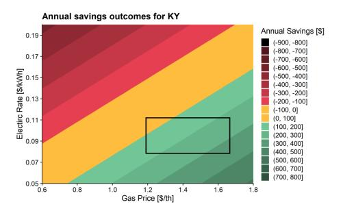
Figure 20: Contour plot of potential savings outcomes for a range of electric and gas rate combinations in Kentucky
