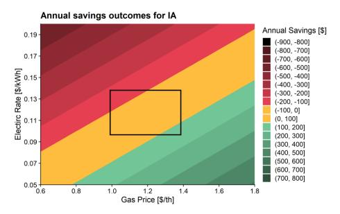
Figure 16: Contour plot of potential savings outcomes for a range of electric and gas rate combinations in Iowa
