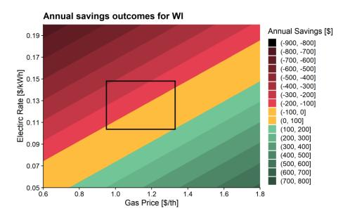
Figure 28: Contour plot of potential savings outcomes for a range of electric and gas rate combinations in Wisconsin
