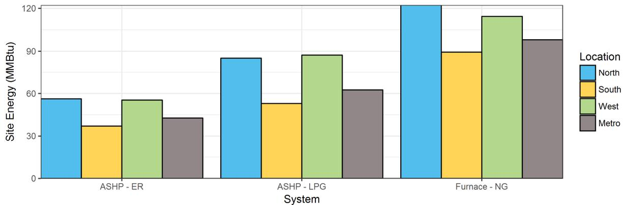
Figure 4: Annual site energy use for space heating of comparable systems
