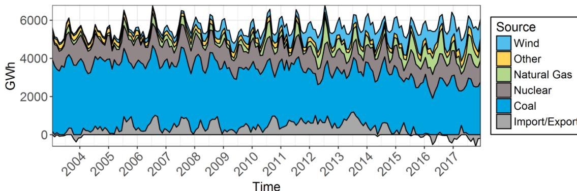
Figure 1: Results of historic monthly production by modified in-state plant
