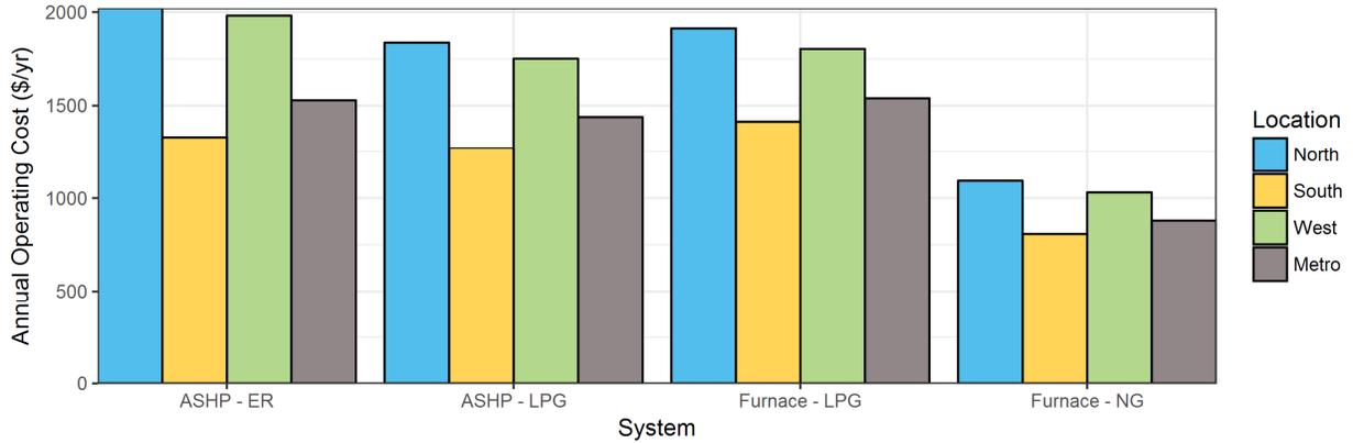
Figure 7: Current annual operating costs for comparable space heating systems
