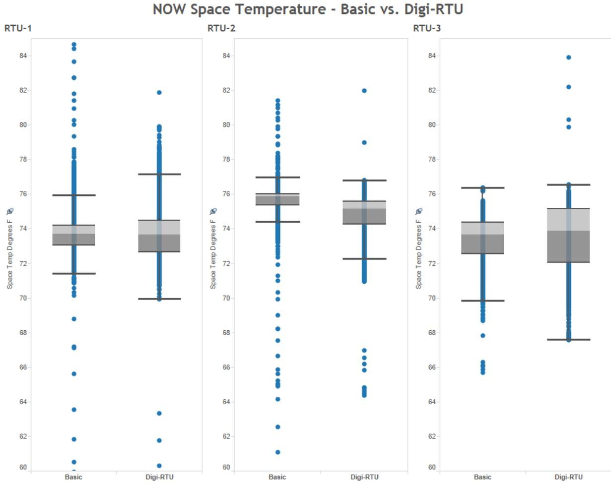
Figure 48. Space temperature box and whisker plots for NUR site (RTUs 1-5)
