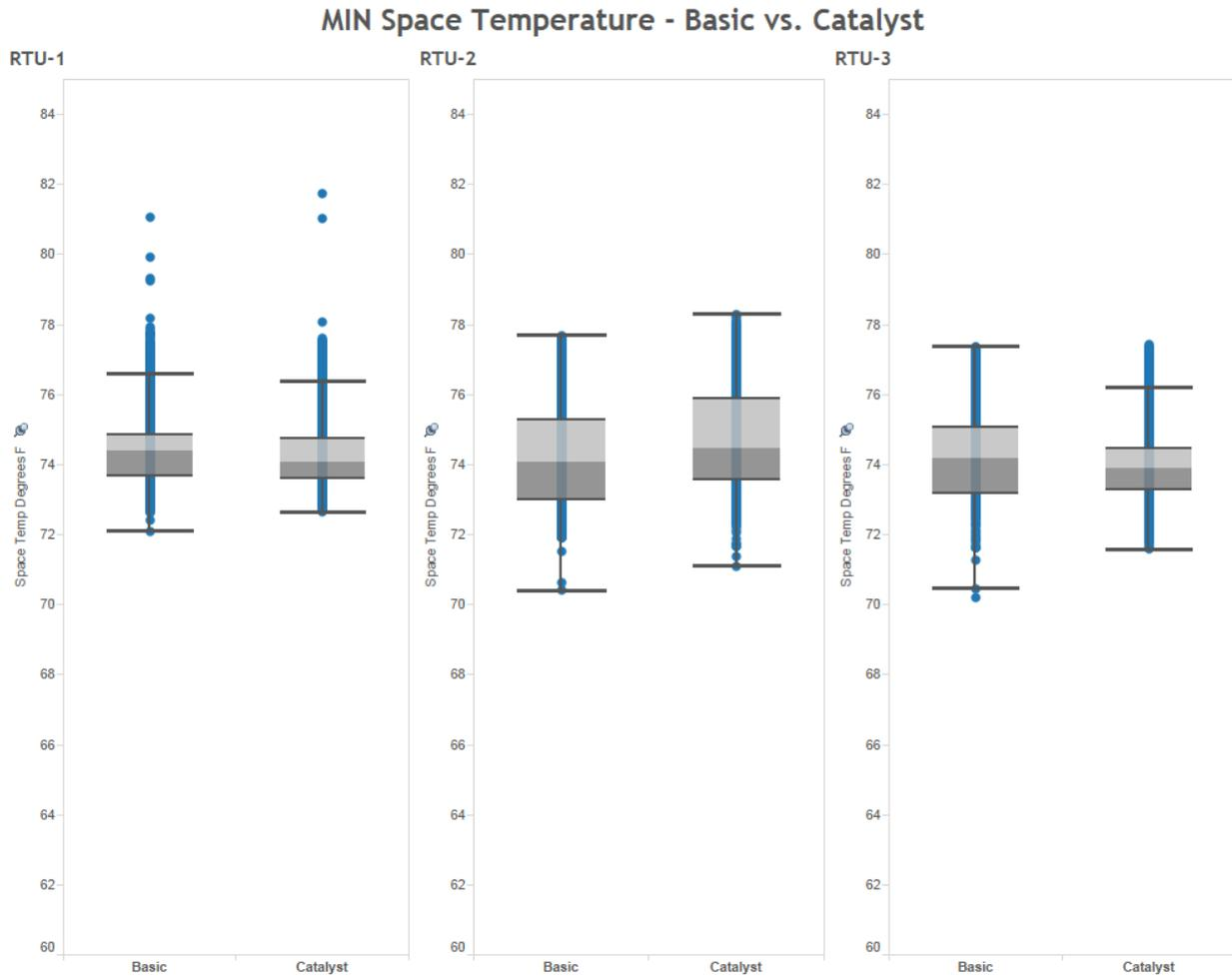
Figure 46. Space temperature box and whisker plots for MIN site (RTUs 4-6)
