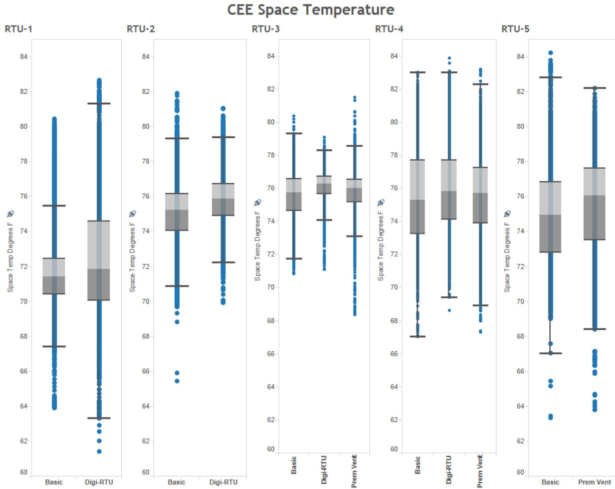
Figure 41. Space temperature box and whisker plots for MDH site (RTUs 1-5)
