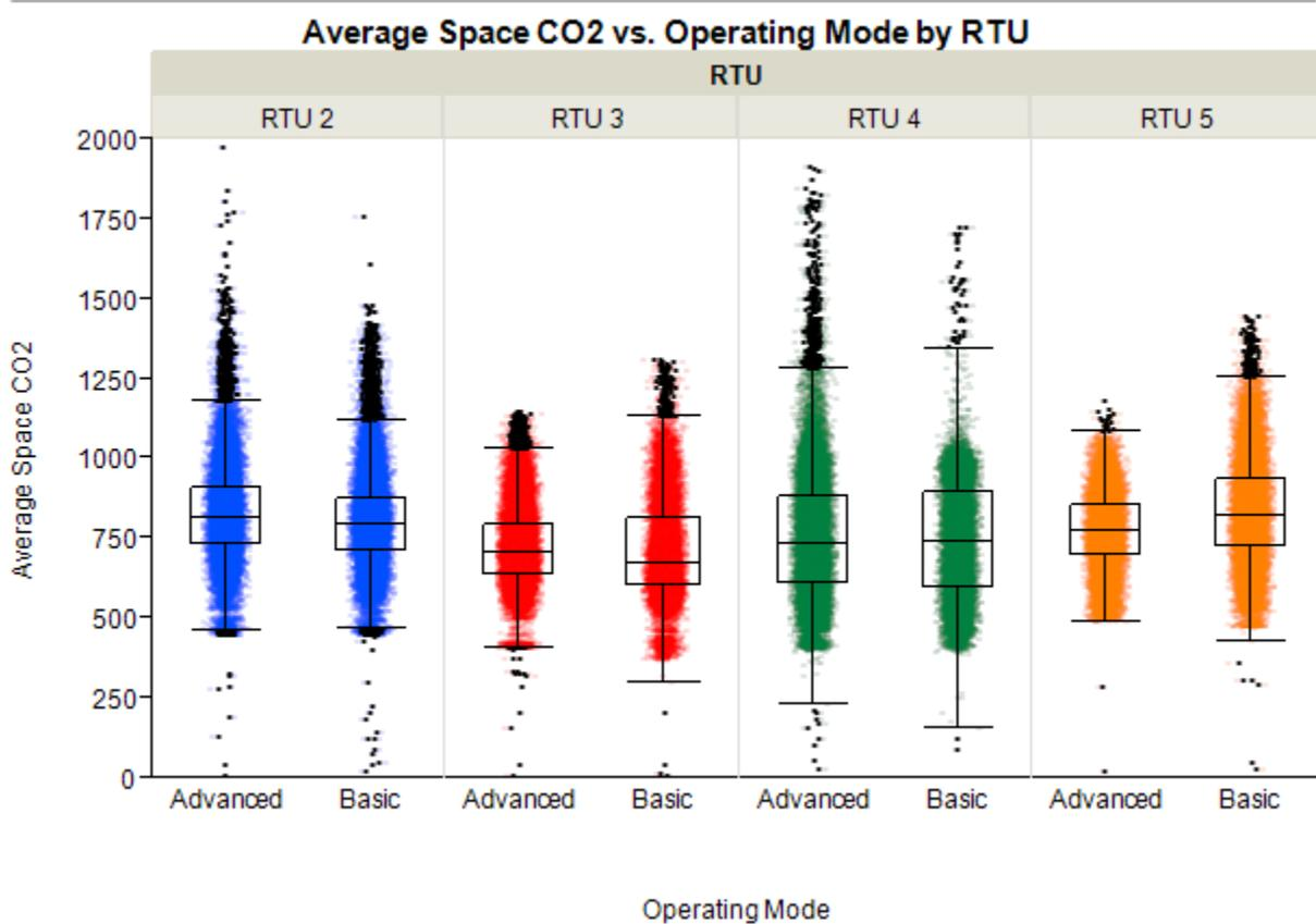
Figure 54. Overall Average Space CO2 Analysis for MIN Units
