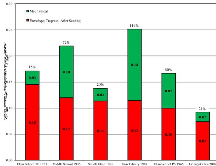
Figure 4: Building normalized envelope and mechanical system leakage
