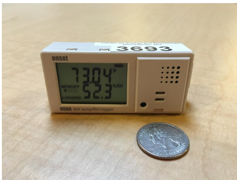
Figure 16. Onset HOBO MX1101 Data Logger
