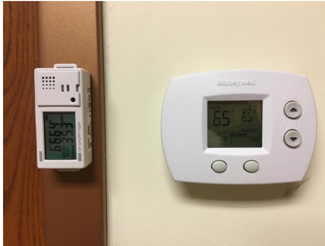
Figure 18. Data Logger Measuring Server Rack Inlet Temperature
