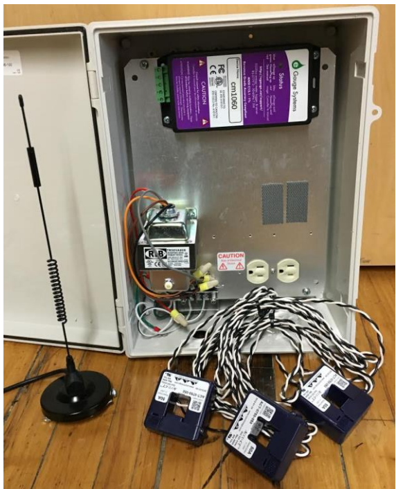
Figure 15. Panel-Installed CT Clamps
