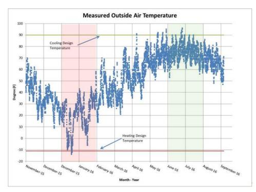
Figure 50 also has lines representing the ASHRAE design outdoor temperatures for the Minneapolis area. From this outside air plot, it is assured that the RTUs did operate at or near the design conditions during the monitoring period.
