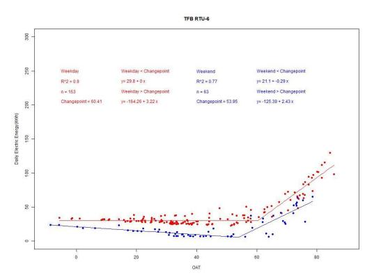
Figure 47 displays a non-typical electric consumption model. There is no difference between the weekday or weekend consumption models as one would expect for a site with a programmable thermostat. This is an office that doesn't have weekend office hours, which should result in lower RTU electric use during the unoccupied periods. The models are slightly different but not enough to assume that the weekend setpoints are different than the weekday.
