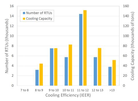
Approximately half (50%) of RTUs with part load cooling efficiencies had an IEER between 10 and 12. For existing RTUs in Minnesota with part load cooling efficiencies, the average IEER is 11.2.
