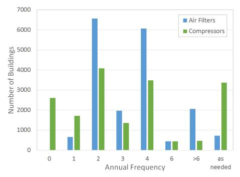
Figure 17: Annual frequency of air filter replacement and compressor cleaning.
