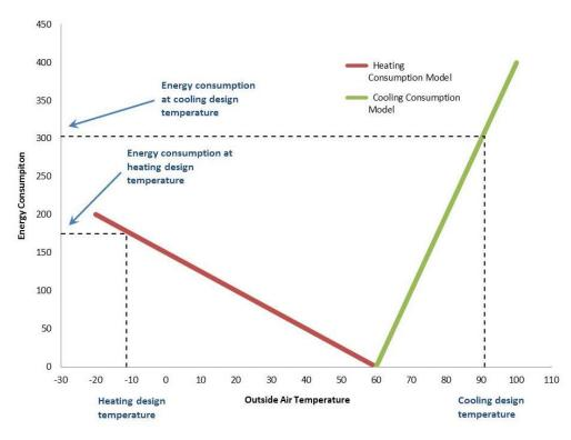
Rated inputs were used as maximum values for capacity for heating and cooling. For the heating season, the rated input for the burner was used as the maximum heat content available to the RTU. With 15-minute data the percent loading for each 15-minute time period is expressed by Equation 5.
