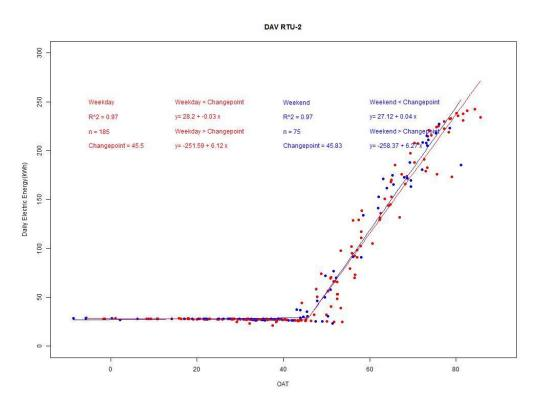
If the economizer were operating correctly for RTU #2 at DAV, there wouldn't be the increase in electric energy at an outside air temperature of 45 degrees. The mechanical cooling on this RTU should be kept off to at least 60, if not 65, degrees outside air temperature, at which time the compressor would need to be utilized to provide cooling to the space.
