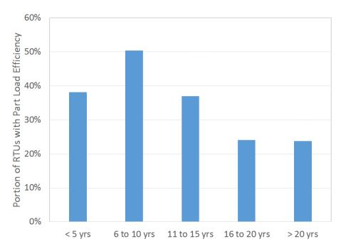
Figure 24: Portion with part load cooling efficiency by RTU age.
