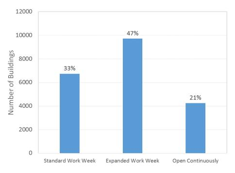
The hours of occupancy affect the RTU energy consumption: longer hours of operation require the RTU to work harder to maintain temperature and humidity setpoints. Figure 13 shows the distribution of weekly occupied hours for buildings served by RTUs throughout Minnesota.
