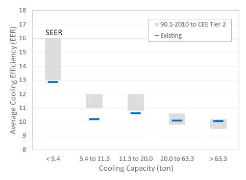
Figure 23: Average cooling efficiency by cooling capacity.
