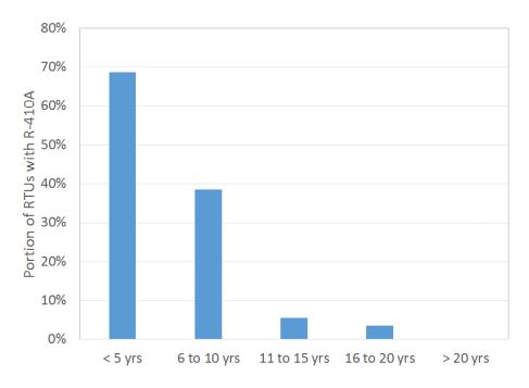
Figure 27: Portion of RTUs with R-410A refrigerant by RTU age.
