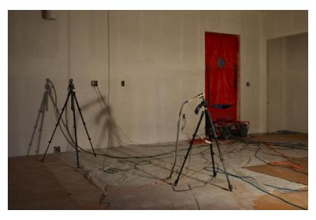
Figure 32. Example of aerosol sealing in a new construction application
