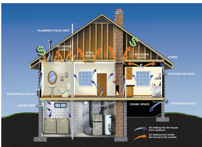
Examples of bypasses or air leaks in your home.
