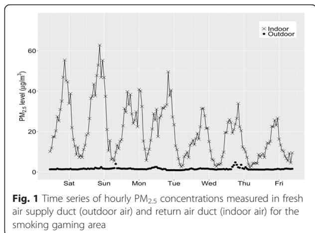
**Fig. 1** Time series of hourly PM<sub>2.5</sub> concentrations measured in fresh air supply duct (outdoor air) and return air duct (indoor air) for the smoking gaming area
