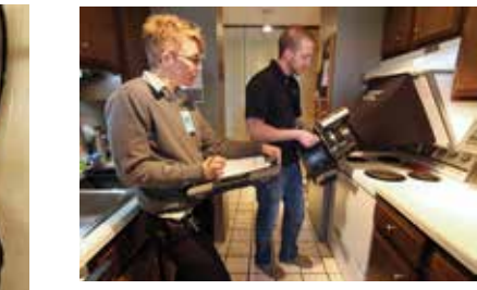
Figure 7: Kitchen inlet measurement. A triangular capture box was constructed so that the FlowBlaster could measure the kitchen range hood flow.
