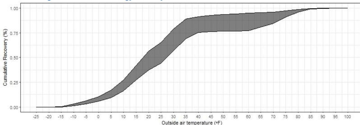
Figure 2 summarizes recommissioned ERV performance using the average recovery energy ratio (RER) for heating and cooling operation. The RER is the ratio of recovered energy to expended energy. There is an energy cost to running an ERV because added fan power is needed to push air through the unit and a motor is sometimes used to spin the unit. The RER offers a performance perspective that allows for a comparison to conventional heating and cooling
