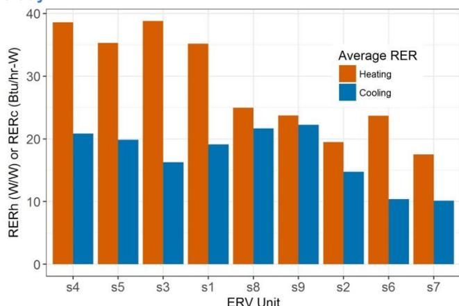
Although heating RER<sub>h</sub> for ERVs are very large at design temperatures (100+ W/W), they are substantially reduced at mild temperatures when there is less recovery. The average heating RER<sub>h</sub> in this study ranged from 17 to 39 W/W, suggesting ERVs are about 20 to 45 times more efficient than gas heating. In this study, these heating RER<sub>h</sub> correspond to heating ventilation load reductions between 34% and 90%.
